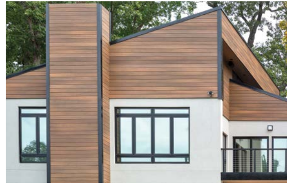
Wood-plastic composites (WPCs) can be used for many different components in the built environment, including decking, soffits, screen facades, rainscreen cladding, and even trim elements when cut to size.
