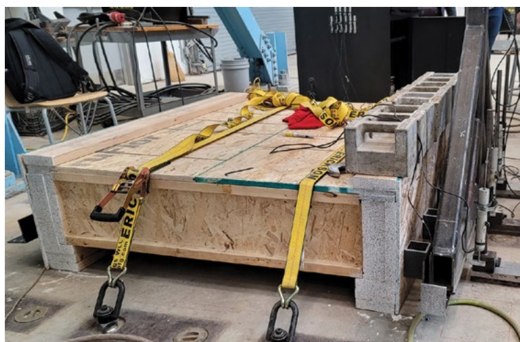
Typical specimen for shelf angles on 102 x 76 x 6.4 mm (3 x 3 x 0.25 in.) fibre-reinforced polymer (FRP) hollow structural sections (HSS) standoffs.
