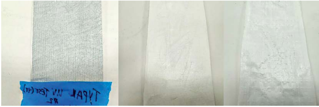
After being exposed to surfactants and subjected to a weathering machine for two days, the left building wrap did not show any damage before or after a scratch test, while the middle and right one both became brittle.
