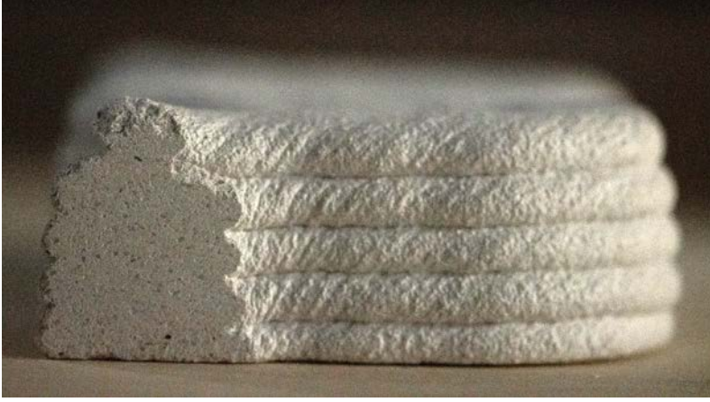
3D concrete printing (3DCP) layer merging.
