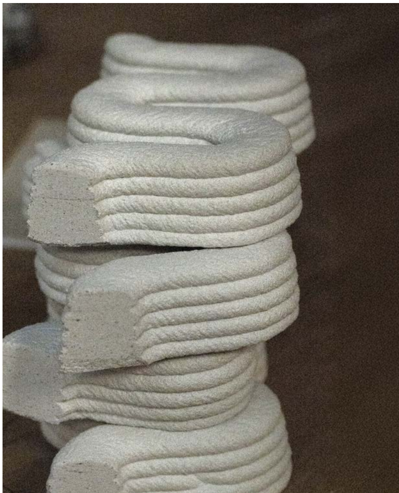
3D printed 2.4-m (8-ft) column.
